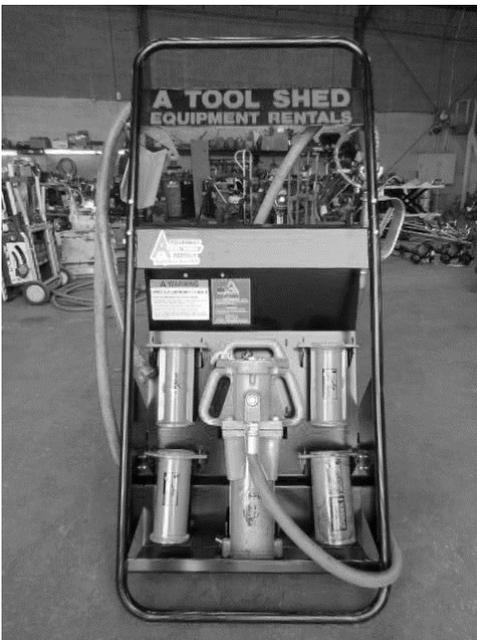
Kit includes: Cart, P-55 Post Driver with Control Handle, 2" 2 1/2" 3" 3 1/2" Post Adaptors, Channel Post Adaptor, Air Oiler/Water Trap with 12' Hose, 1 quart of Oil for the Oiler and two 1/2-13 x 1 1/2" bolts with compression washers.
