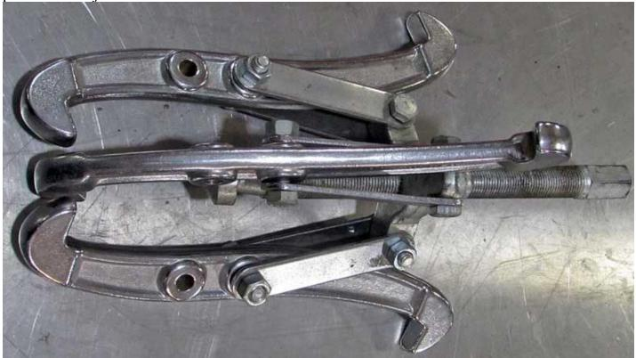
The classic 3-jaw puller works for gears, pulleys and all other manner of press-fit parts that may need some help coming off. Just be careful because they tend to pop loose.
