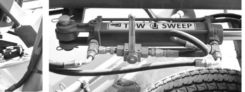
6. Remove the Broom Ram Blocker & use Lock Pin to attach it to the spray pipe.
