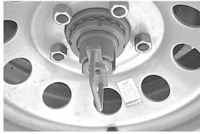
2. Lower the tongue & lock in place with <u>Pin & Clip.</u>
