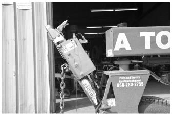
3. Push down the Parking Brake to disengage it.
