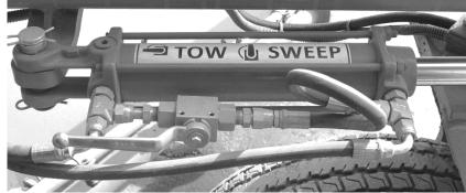
6. Use the Broom Ram Blocker & Lock Pin to hold the brush in the upright position.
