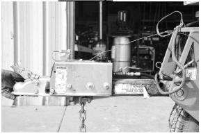
4. Push down the Parking Brake to disengage it
