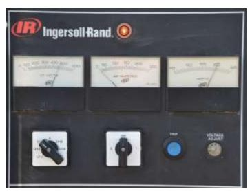
The panel selector switches show how much Voltage and Amperage is being generated between each lug. **Note:** The amp meter will only register when there is a load hooked to the generator.
