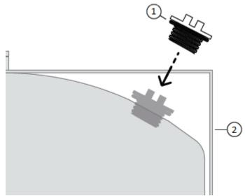
When installing the plug (#1 in figure above) note that there is an O-ring, ensure O-ring properly seats against the roller. A portion of the plug will extend from the roller, however, it will not interfere with the scraper bar (#2 in figure above)
