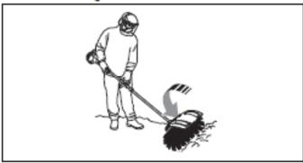
In order to get into corners, remove the splash guard and loosen the accessory coupling and rotate the accessory half a turn.
