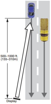
**Correct Positioning:** Angled slightly toward the roadway, the drivers have a long viewing distance.
