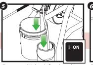
Turn power ON. Steady flow through the return tube for 5 seconds
