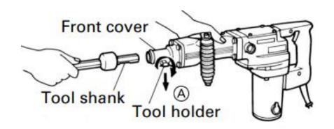
How to install a tool, ie: the bit:
