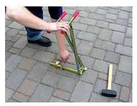
3. Next, insert the QUICK PIN. The holes on the slide and bar are offset for precise handle width. The width should allow both handles to be squeezed with one hand without touching when force is applied.
