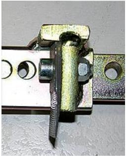
WARNING Improper use of this tool will bend the teeth straight. This item is not covered by the Equipment Protection Plan. Note: this picture shows the proper curve of a tooth.
