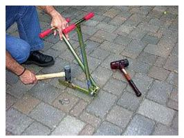
2. When it is time to set-up the PAVEREXTRACTOR, first remove the QUICKPIN. Then line up the teeth with the joint and hammer both ends down until the frame is tight to the top of the paver. It is critical that the teeth are down as far as possible.
