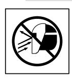
Arc rays from the welding process produce intense visible and invisible (ultraviolet and infrared) rays that can burn eyes and skin. Sparks fly off from the weld.
